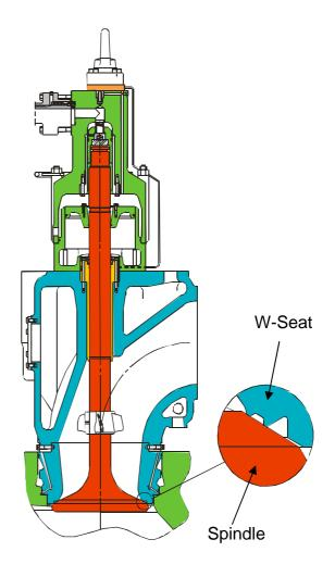
Extended service tests with the W-seat (logging up to 40,000 service hours) and standard MAN B&W hard facings, including Nimonic 80A on the spindle, have shown that the necessary overhauling/grinding of the seat is reduced to a minimum, and that it can be carried out as a routine job during regular docking of the vessel.
